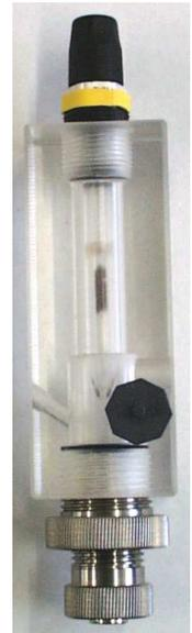
The working electrode  $E_A$  (8) consists of large-area gold round blank (8a), inserted in the electrode holder (8b). This assembly is screwed from the bottom into the measuring cell. Blue glass beads moved by the measuring water are cleaning the surface of the gold electrode. The reference system (12) made of an Ag/AgCl electrode with the ring-shaped counter electrode made of gold is screwed into the measuring cell from above. This electrode is marked by a yellow ring.
